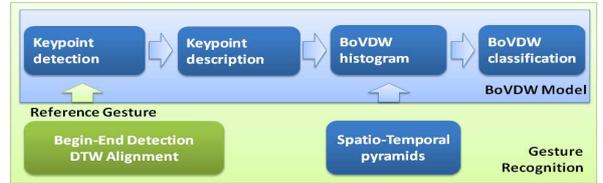
Figure 2. BoVDW-based Gesture Recognition.
